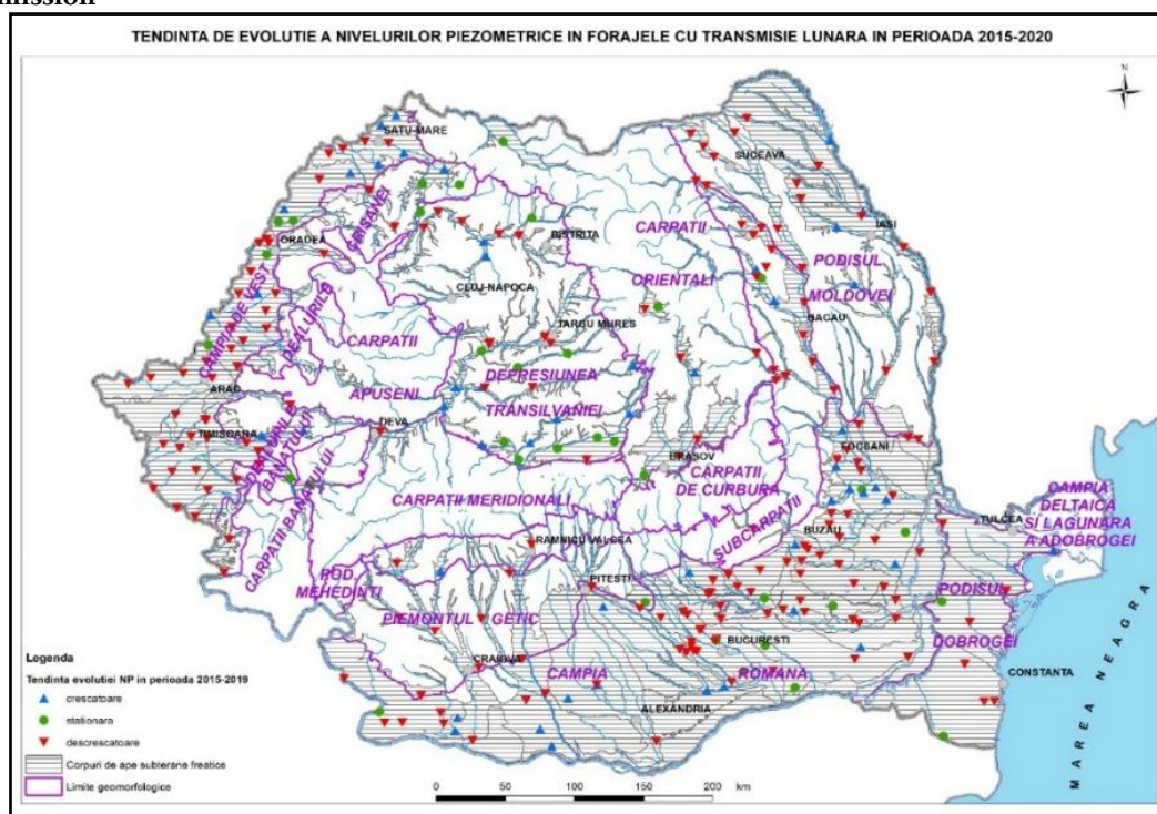
Figure II.3 Trend in the evolution of monthly piezometric levels (NP) in the period 2015-2020-monitoring boreholes for monthly transmission
